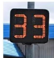
The “advanced” SID displays the speed of approaching vehicles and displays a “Slow Down” message to vehicles exceeding the speed limit. This is slightly larger but is much heavier, weighing 12kg plus a 12kg battery. The battery life is also significantly reduced.
